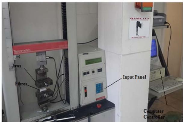
Fig.4 Testometric micro 500 used for fibre tenacity testing
