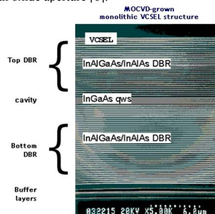
FIG.2 THE STRUCTURE OF THE RAYCAN VCSEL [7]
