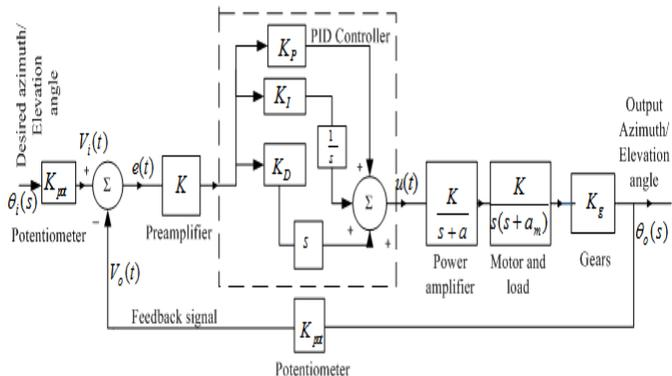
Fig.4 Block diagram of Antenna Azimuth PID controller.
