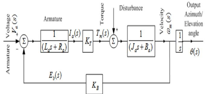
Fig.3 Block diagram of separately excited DC servomotor
