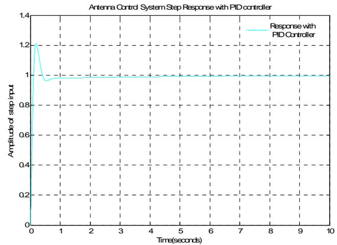
Fig.8 Step response of system with PID controller
