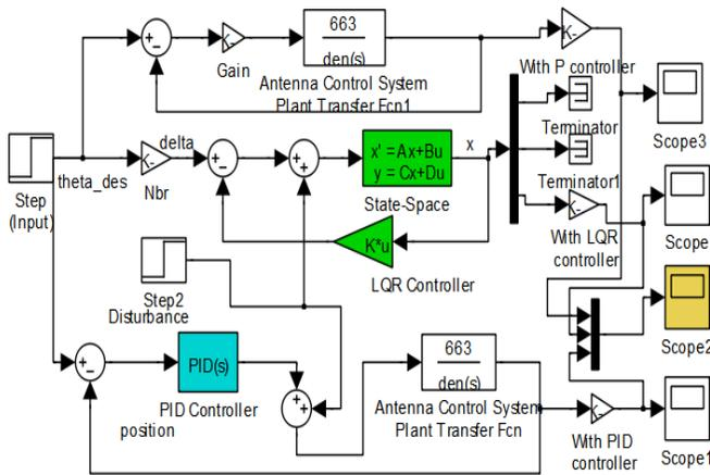
Fig.6 PID & LQR Control Simulink model layout
