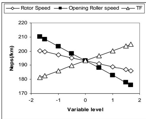
Fig.1 The effect of single variables on Neps/km
