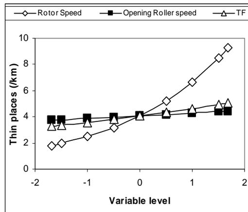
Fig. 9: The effect of single variable on thin places/km
