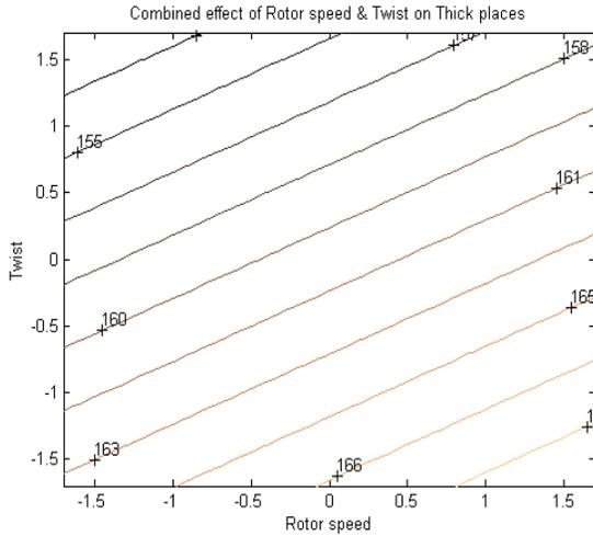
Fig. 7: Combined effect of rotor speed and twist on thick places
