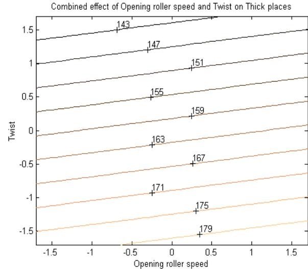
Fig. 8: Combined effect of opening roller speed and twist on thick places
