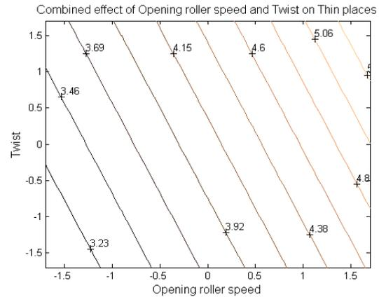
Fig. 12: The combined effect of opening roller speed and twist on thin places
