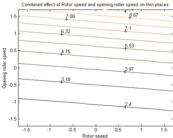
Fig. 10: The combined effect of rotor speed and opening rollers speed on thin places/km
