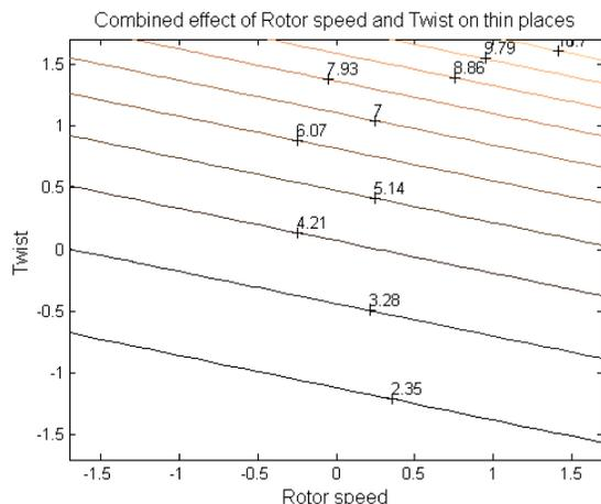
Fig. 11: The combined effect of rotor speed and twist on thin places/km
