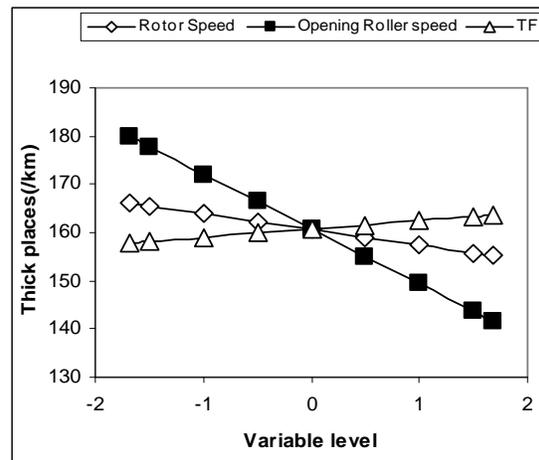
Fig. 5: The effect of singles variables on thick places/km
