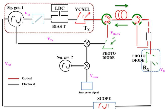
Fig. 2 Block diagram illustrating the simulated electro-optic frequency dissemination system
