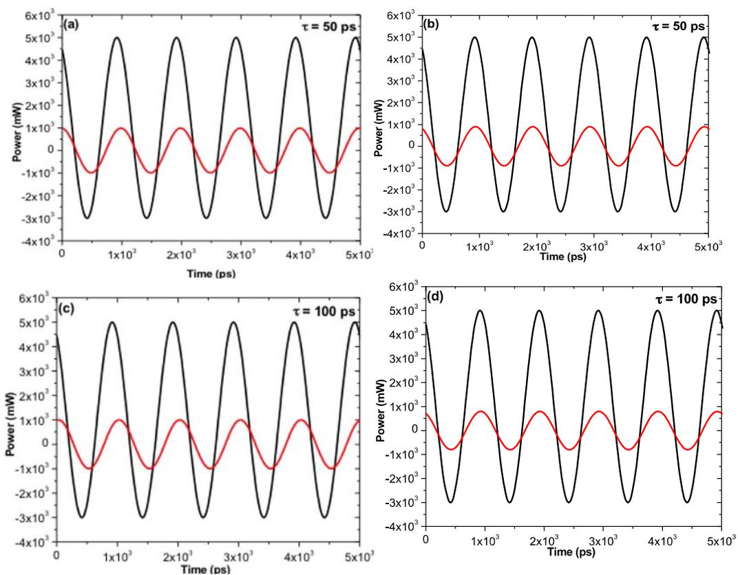
Fig. 4 Illustration of the relative phase shift between the reference signal  $V_{ref}$  and the received signal  $V_{Rx}$  before and after the phase offset is applied. 50 ps and 100 ps induced fibre delays were employed as shown in (a), (b) and (c), (d) respectively.
