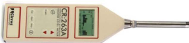
**Plate 2:** An Integrating Sound Level Meter
