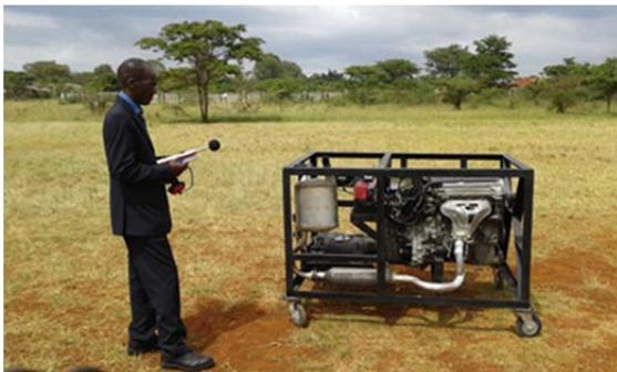
Plate 3: Noise sampling with Exhaust Piping in place
