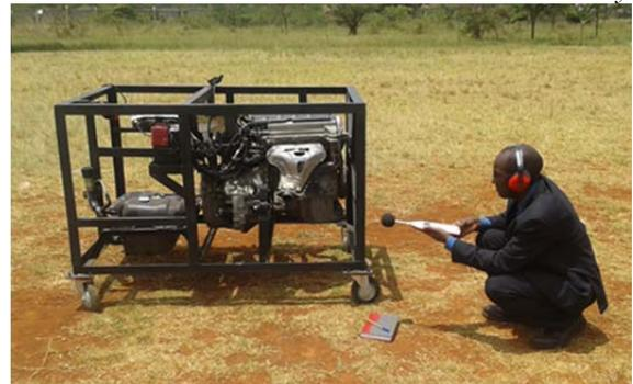
Plate 4: Noise sampling with Exhaust Piping removed
