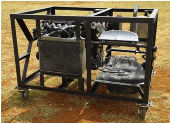
**Plate 1:** A 1500cc VVT-i gasoline engine noise source
