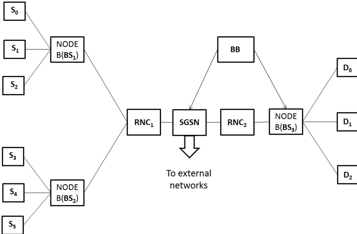
Figure 1: Simulation Model for an IP-based Radio Access Network of UMTS network with Bandwidth Blocker
