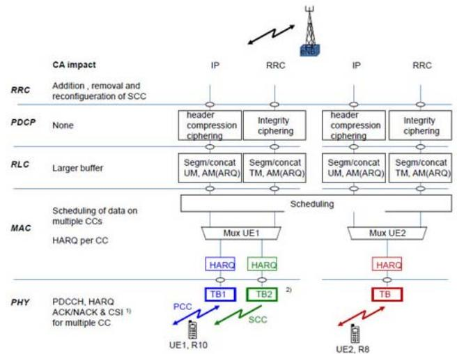
Fig. 3 Radio Interface LTE protocols, with CA Introduction [22]
