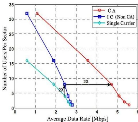
Fig. 5 (b) Throughput performance of CA, Independent Carrier and Single Carrier Scheduler for Burst Traffic [31]
