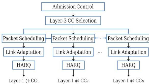
Fig. 2 Structure of RRM for LTE advanced with Carrier Aggregation Support [21]
