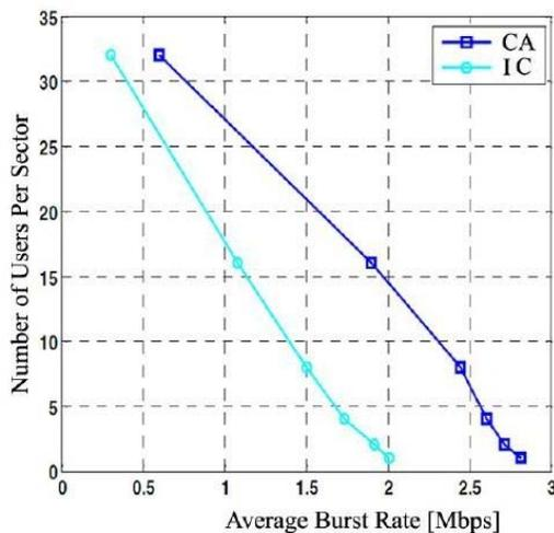
Fig. 5 (a) Throughput performance of CA and Non-CA Independent Carrier Scheduler for Burst Traffic [31]
