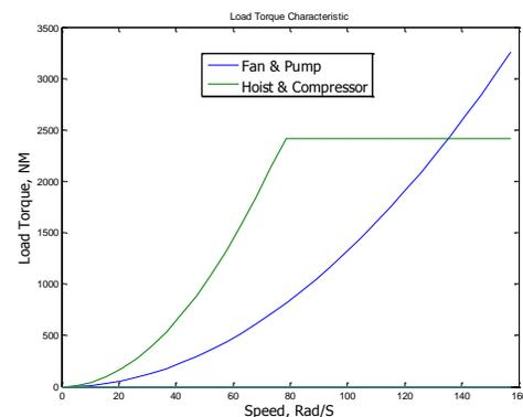
Figure 2: Load Torque Characteristics
