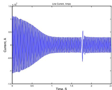
Figure 3: Total Line Current, Phase A
