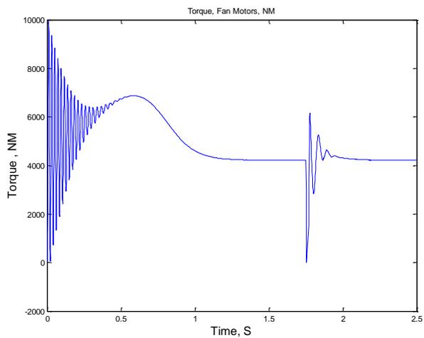
Figure 6: Electromagnetic Torque, Aggregated Fan & Pump Motor
