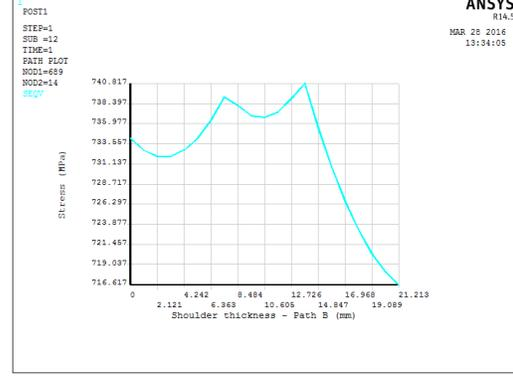
Fig. 37. Von Mises stress on path B - Plastic model with nozzle:  $r_c = 80mm$
