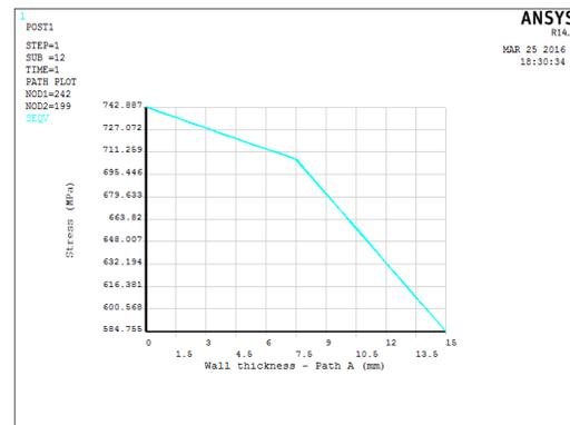
Fig. 27. Von Mises stress on path A - Plastic model without nozzle:  $r_c = 80mm$
