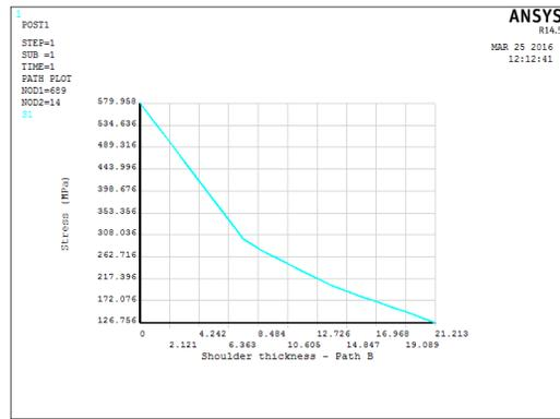
Fig. 21. Hoop stress on path B - Elastic model with nozzle
