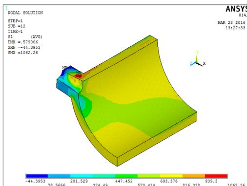
Fig. 34. Hoop stress - Plastic model with nozzle:  $r_c = 80mm$
