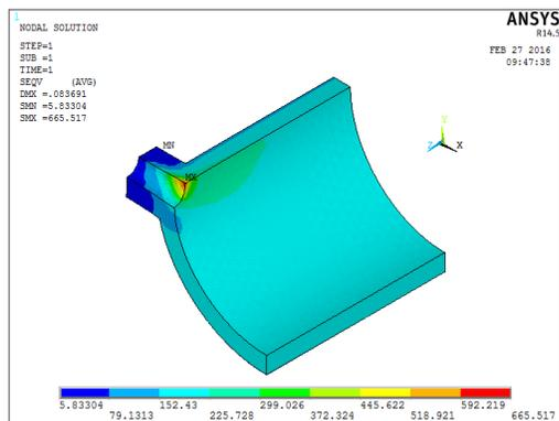
Fig. 20. Von Mises stress - Elastic model with nozzle
