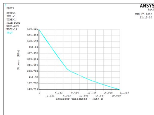
Fig. 22. Von Mises stress on path B - Elastic model with nozzle
