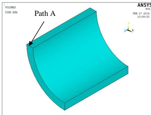
Fig. 5. An eighth section model without nozzle
