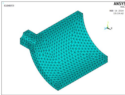
Fig. 10. Meshed model with nozzle
