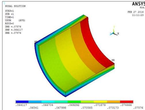
Fig. 18. Resultant displacement - Elastic model without nozzle
