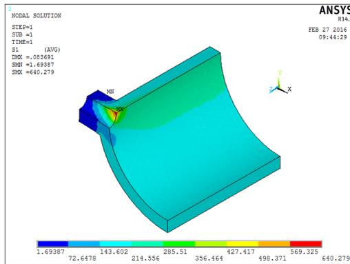
Fig. 19. Hoop stress - Elastic model with nozzle
