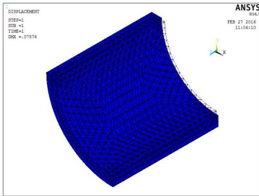
Fig. 17. Deformed shape - Elastic model without nozzle
