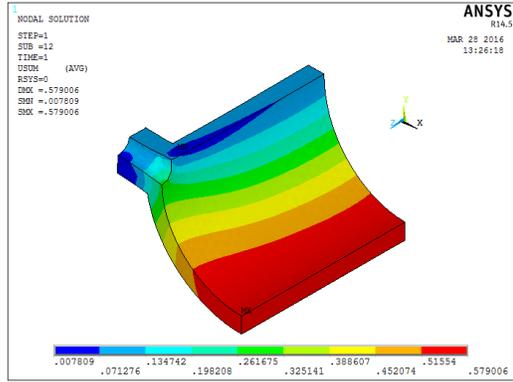
Fig. 38. Resultant displacement - Plastic model with nozzle:  $r_c = 80mm$
