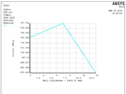
Fig. 26. Hoop stress on path A - Plastic model without nozzle:  $r_c = 80mm$
