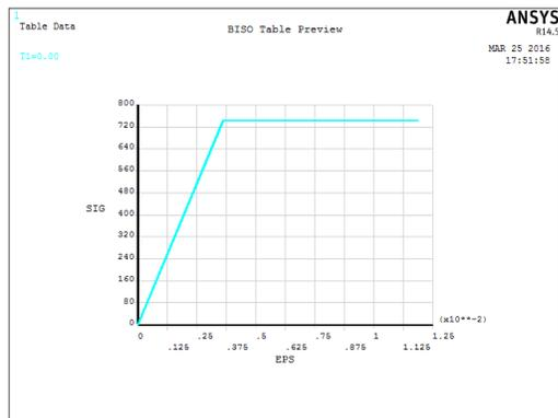
Fig. 11. FE plastic stress-strain curve without strain hardening
