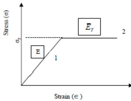
Fig. 4. Stress-strain curve without strain hardening
