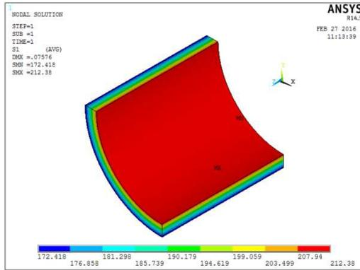
Fig. 12. Hoop stress - Elastic model without nozzle
