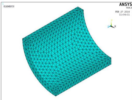
Fig. 7. Meshed model without nozzle
