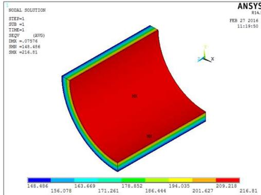
Fig. 13. Von Mises stress - Elastic model without nozzle
