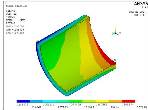
Fig. 28. Resultant displacement - Plastic model without nozzle:  $r_c = 80mm$
