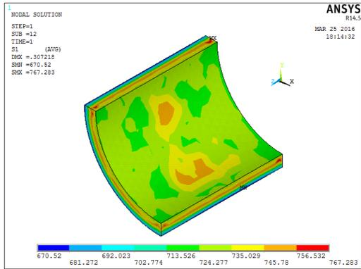
Fig. 24. Hoop stress - Plastic model without nozzle:  $r_c = 80mm$
