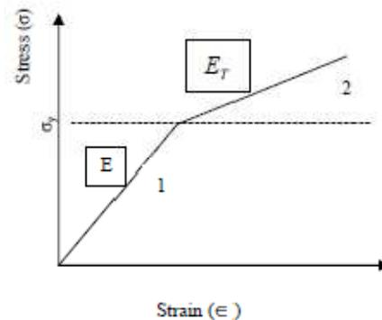
Fig. 3. Stress-strain curve with strain hardening
