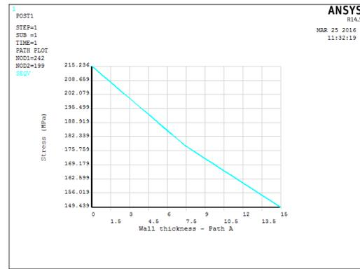
Fig. 15. Von Mises stress along path A - Elastic model without nozzle
