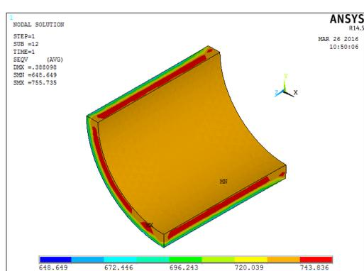
Fig. 30. Von Mises stress - Plastic model without nozzle:  $r_c = 85mm$
