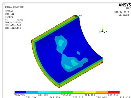
Fig. 29. Hoop stress - Plastic model without nozzle:  $r_c = 85mm$
