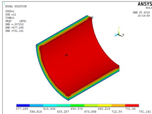
Fig. 25. Von Mises stress - Plastic model without nozzle:  $r_c = 80mm$
