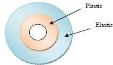
Fig. 2. Elastic-plastic region across the wall thickness
