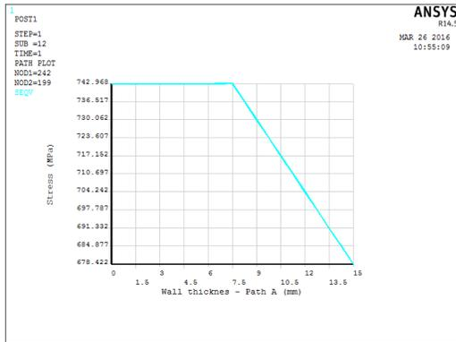
Fig. 32. Von Mises stress on path A - Plastic model without nozzle:  $r_c = 85mm$
