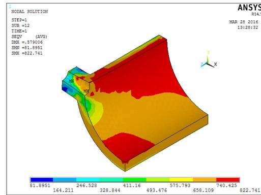
Fig. 35. Von Mises stress - Plastic model with nozzle:  $r_c = 80mm$
