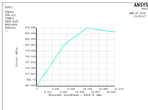
Fig. 36. Hoop stress on path B - Plastic model with nozzle:  $r_c = 80mm$
