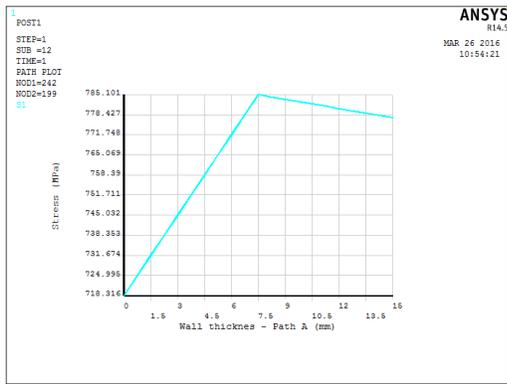
Fig. 31. Hoop stress on path A - Plastic model without nozzle:  $r_c = 85mm$
