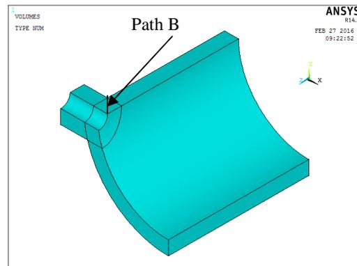
Fig. 8. An eighth section model with nozzle
