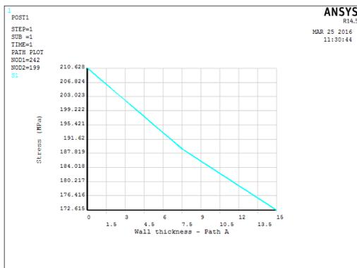
Fig. 14. Hoop stress along path A - Elastic model without nozzle
