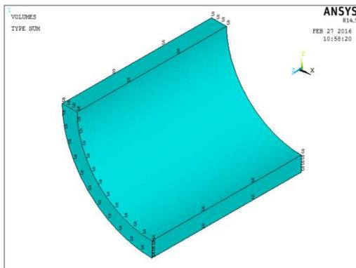
Fig. 6. Boundary condition areas on model without nozzle
