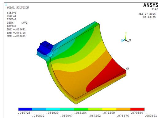
Fig. 23. Resultant displacement - Elastic model with nozzle
