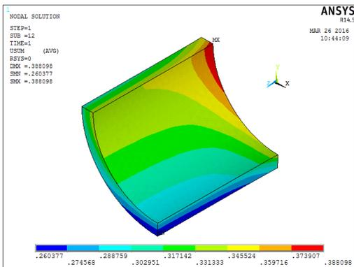
Fig. 33. Resultant displacement - Plastic model without nozzle:  $r_c = 85mm$
