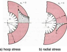
Fig. 1. Hoop and radial stress distribution within the pressure vessel wall
