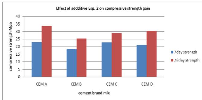
Figure 9: Effect of Esp 2. Plant Extract on Compressive Strength
