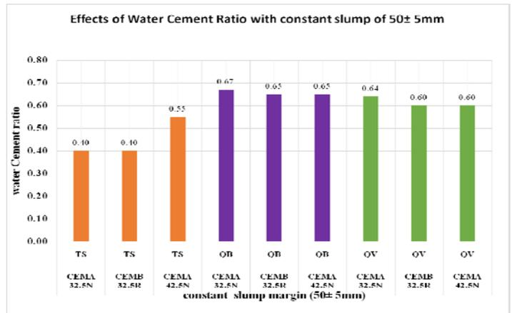
**Figure 3: Effect of Fine aggregates type and cement type on the Water/ Cement Ratio Results**
