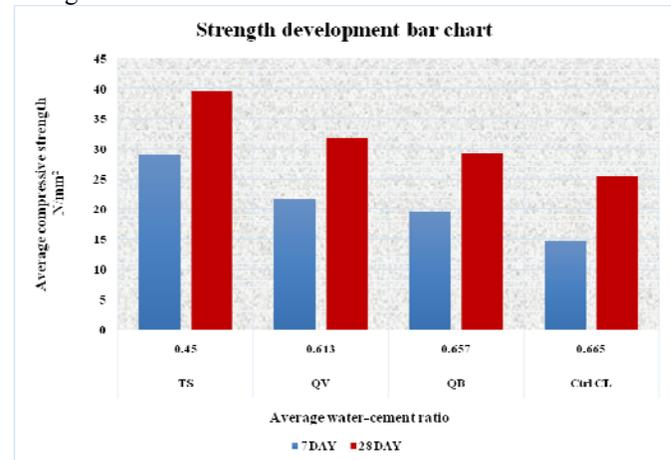
Figure 6: The Relationship between the Water/Cement Ratio and the Compressive Strength
