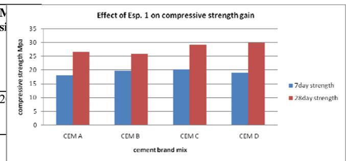
**Figure 8: Effect of Plant Extract on Compressive Strength**
