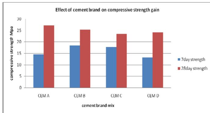
**Figure 7: Effect of Cement Brand on Compressive Strength**
