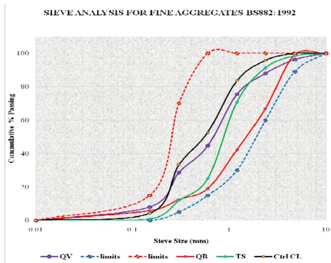
**Figure 1: Sieve Analysis Results for the Fine Aggregates**
