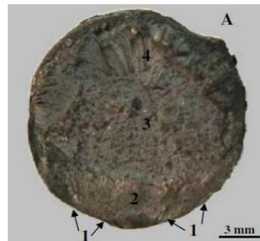
Fig. 3 Fatigue Crack Propagation
