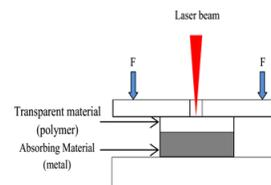
Fig. 2. A typical laser joining system.
