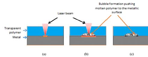
Fig. 1. Sequence of laser joining mechanism
