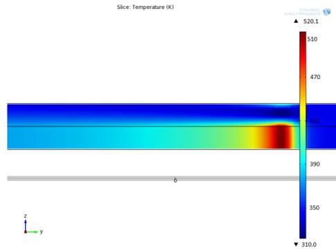
Fig. 6. Temperature Contour at the (Y-Z) plane at time 1 s
