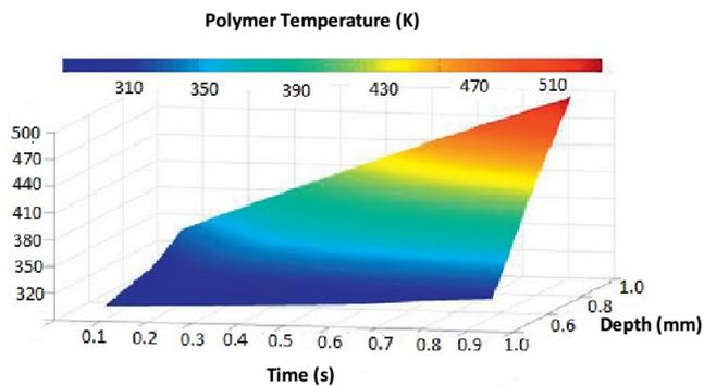
Fig. 8. Temperature Distribution on the interface along the irradiation path
