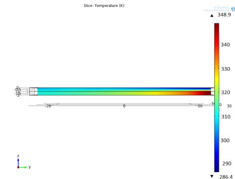
Fig. 7. Temperature Contour at the (Y-Z) plane at time 2 s
