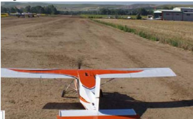
Fig.2 Quanta-G fixed wing UAV (Quantalab, Spain)
