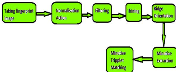
Fig 2. Fingerprint Image Processing by Minutiae Technique
