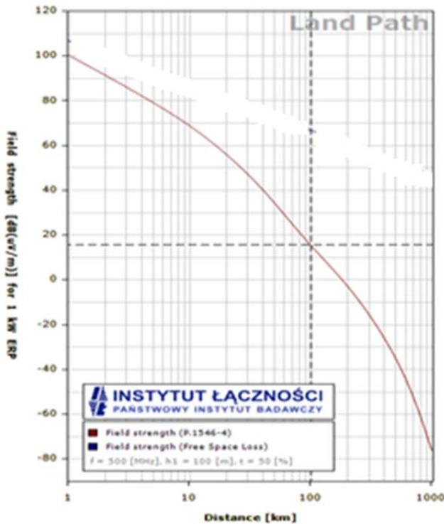
Fig.4 Field Strength for 500 MHz
