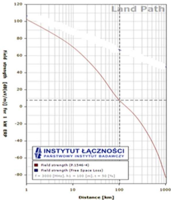
Fig.5 Field Strength for 3000 MHz
