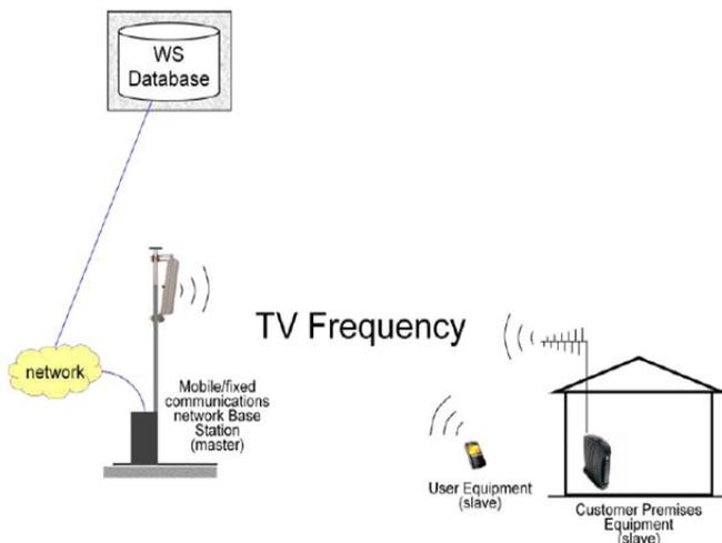
Fig. 3 Typical TVWS network setup
