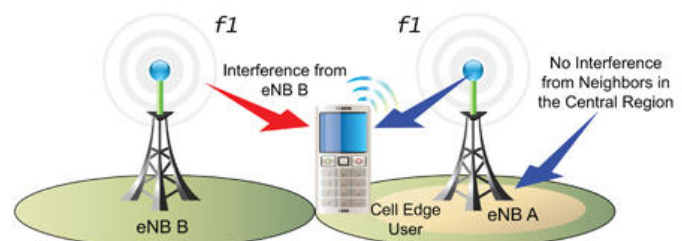
Fig. 1 A demonstration of Inter-cell interference in an LTE system [2]
