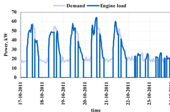
Fig. 6. Demand vs optimal engine load
