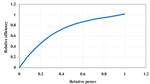
Fig. 1. Relative engine efficiency (based on [39])
