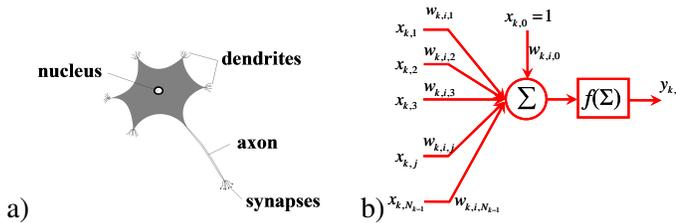
Fig. 3. Neuron scheme (a) and its mathematical model (b) [40]
