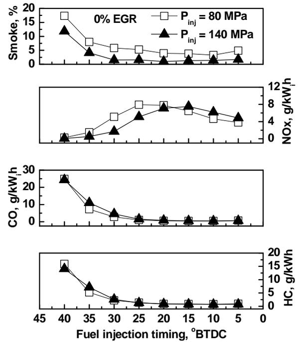
Fig.4. Effect of injection pressure on specific emissions
