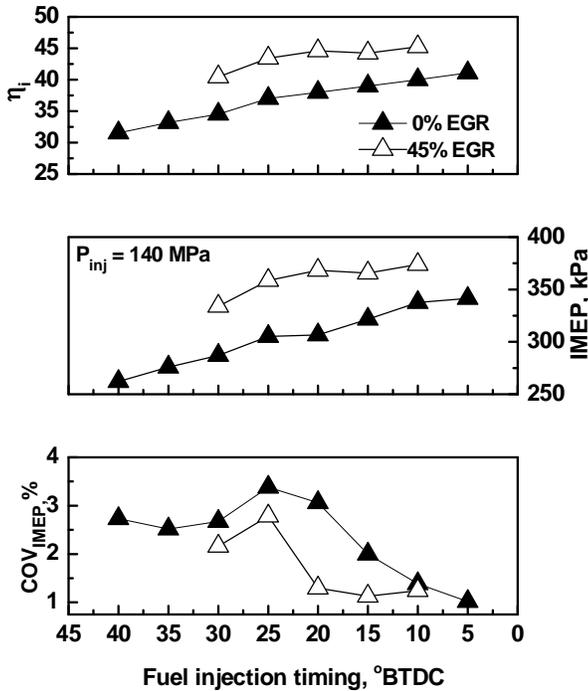
Fig.9. Effect of EGR on indicated thermal efficiency, IMEP and COV<sub>IMEP</sub>
