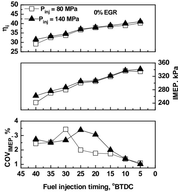
Fig.3. Effect of injection pressure on indicated thermal efficiency, IMEP and COV<sub>IMEP</sub>
